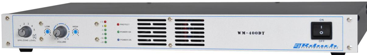
WM-DT acoustic amplifiers are equipped with a class D amplifier 0dB and +6dB symmetrical inputs, 0dB output, gain control, soprano and bass control, limiter and 6-degree controlling indicator. The input has a Combo type socket, which allows connecting the signal by means of a wire with XLR or Jack plug. Modern construction of WM-DT amplifiers lets them cooperate with other amplifiers and mixer in order to increase the power of the entire amplification installation.
